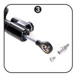
Now mount the steering damper **6** to the lamp bracket **8** and to the frame part **7** between the footboard and the handlebar.
