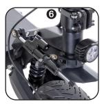
Finally, set the handlebars all the way to the left and then tighten the adjusting screw **9** firmly. The strength can now be adjusted on the adjusting wheel above the steering damper.
