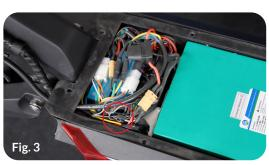
In the cable shaft there are 2 black connectors with black/ white cables (Fig. 3, 4).
